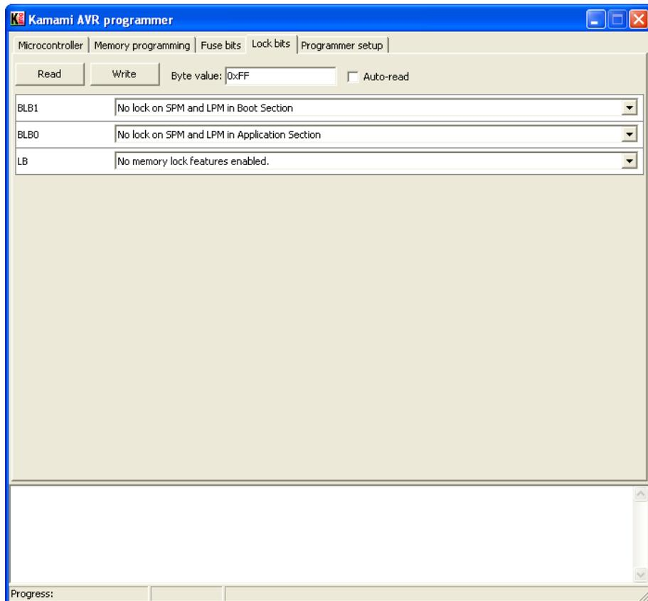
*Fig. 6. Lock bits tab of KamPROG for AVR application*
